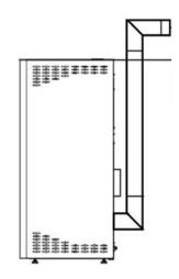
It is compulsory to connect the appliance to a chimney that is suitable for solid fuels. The pipes from the oven to the chimney must be made of metal. It is also of importance to contact your chimney sweeper. When more stoves are connected to the one chimney the chimney sweeper must be consulted. The pressure (chimney draught) must be approximately between 6 and 15 PA. Our appliances are programmed for an average pressure, but the engineer can adjust this correctly when installing the appliance.
